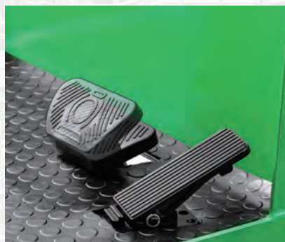
Large Brake Pedal with Integrated Parking Brake Design
